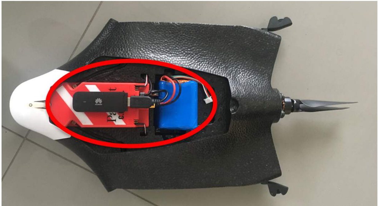
Figure 2: 4G module installed on the Parrot Disco UAS
