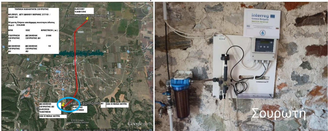
Figure 3.2.10. Map of boreholes and tanks in Souroti – tank Δ1 (where automated chlorination system is installed) is shown in circle
