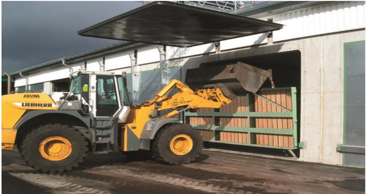
Fig. 6. Charging a bioreactor with a front loader
