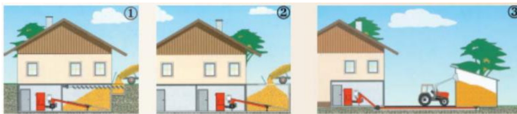
Figure 10: Storage and transport of biomass fuel at the refueling point (TEE, 2011)
