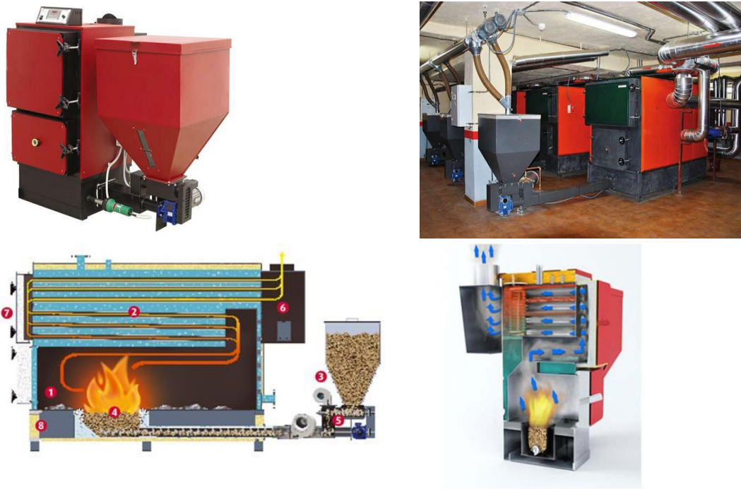
Figure 9: Biomass boiler (agroenergy, 2022)
