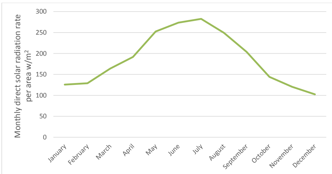
Diagram 2.6 – Monthly site direct solar radiation rate per area W/m² of C. Xenakis Museum
