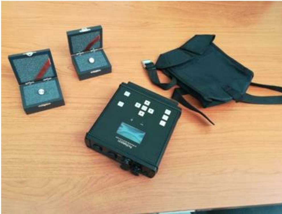
Figure 7. Pettersson ultrasound recording unit
