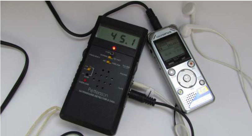
Ultrasound detector for bats with recording device
