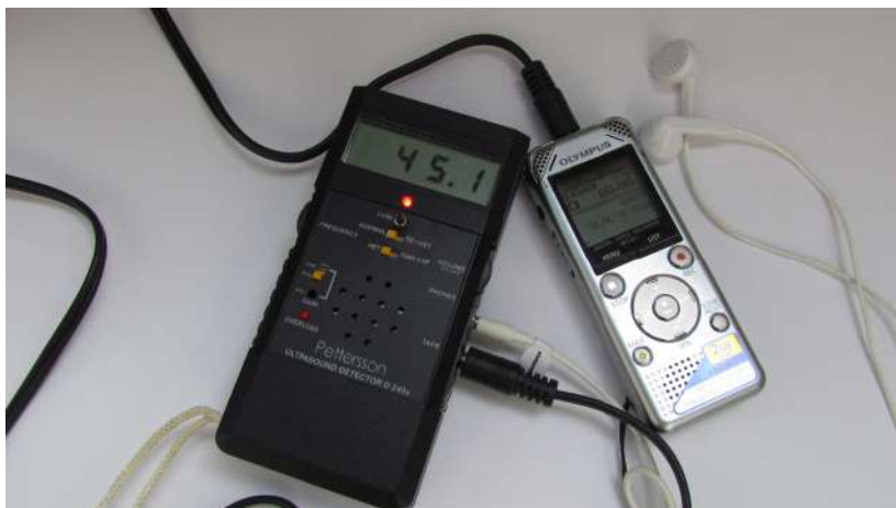
Ultrasound detector for bats with recording device
