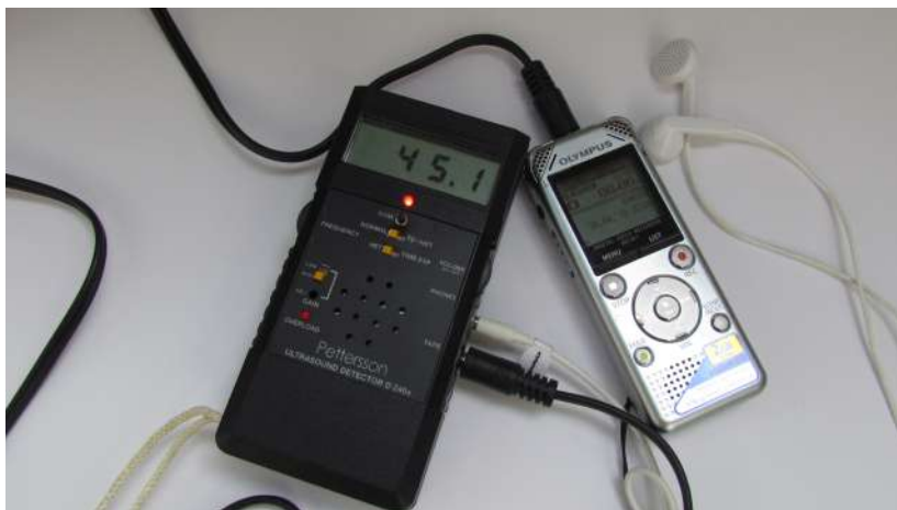
Ultrasound detection for bats that is recording
